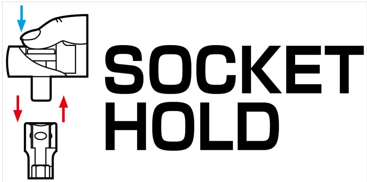
Figure 1: Socket Hold Mechanism. This diagram shows how to engage and disengage a socket from the ratchet head using the push-button release.
