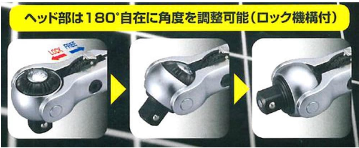
Figure 5.1: A sequence of images demonstrating the 180-degree swivel capability of the ratchet head and its locking mechanism for secure positioning. Slide the lever to 'FREE' to adjust the angle, then to 'LOCK' to secure it.
