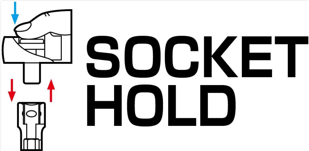
Figure 4.1: A visual guide demonstrating how to attach and detach sockets using the socket hold mechanism, ensuring secure connection.
