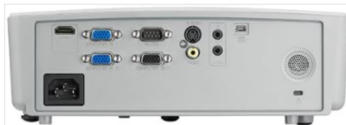
Figure 4.3: Rear panel of the Vivitek D555 projector showing various input and output ports. These include HDMI, dual VGA inputs, VGA output, S-Video, Composite Video, audio input/output, and a USB port.
