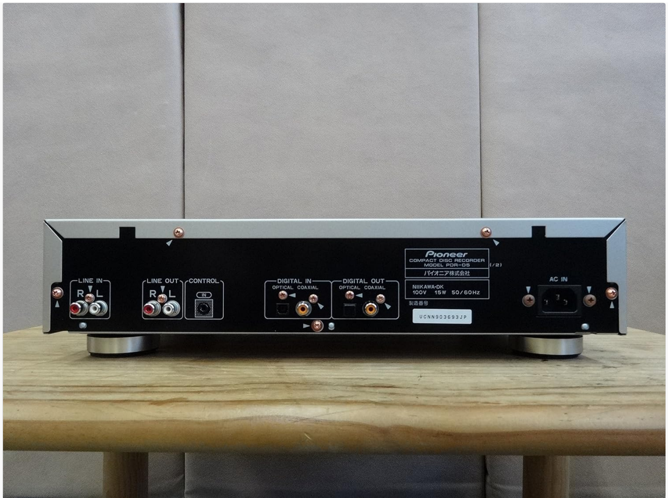
Image: The rear panel of the Pioneer PDR-D5 CD Recorder, illustrating the LINE IN, LINE OUT, DIGITAL IN (Optical/Coaxial), DIGITAL OUT (Optical/Coaxial), and AC IN connections.
