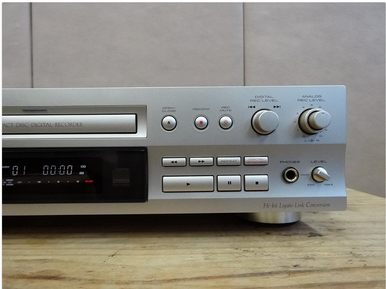
Image: The front right section of the Pioneer PDR-D5 CD Recorder, displaying the OPEN/CLOSE, RECORD, REC MUTE, DIGITAL REC LEVEL, ANALOG REC LEVEL, PLAY, PAUSE, STOP, SKIP, REPEAT, DIGITAL SYNC, PHONES, and LEVEL controls.
