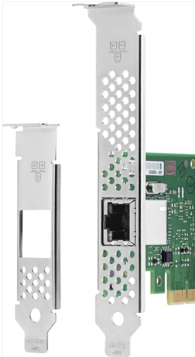
Figure 3.1: Intel I210-T1 Network Adapter with included full-height and low-profile brackets. The main adapter board is green with gold PCIe contacts, and the brackets are silver-colored metal.
