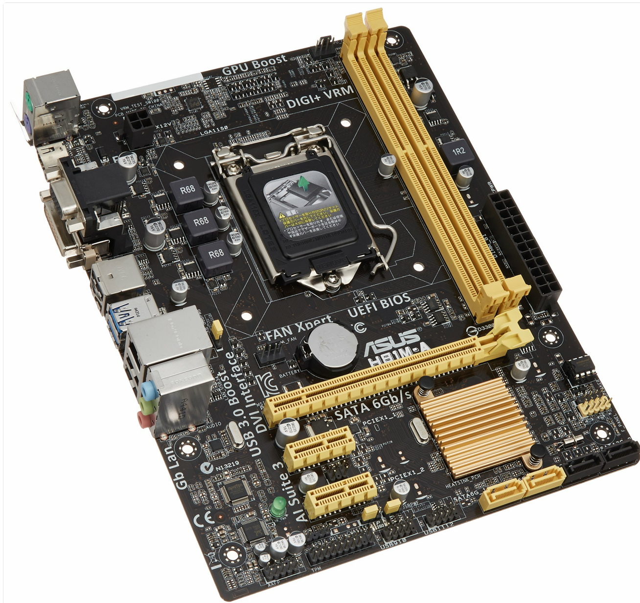
Figure 5.1: Rear I/O panel of the ASUS H81M-A motherboard, showing PS/2 ports, VGA, DVI, HDMI, USB 2.0, USB 3.0, LAN, and audio jacks.
