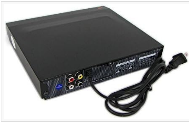
Figure 4.2: Rear view of the QFX VP109BLK player, highlighting the audio/video output ports and power input.
