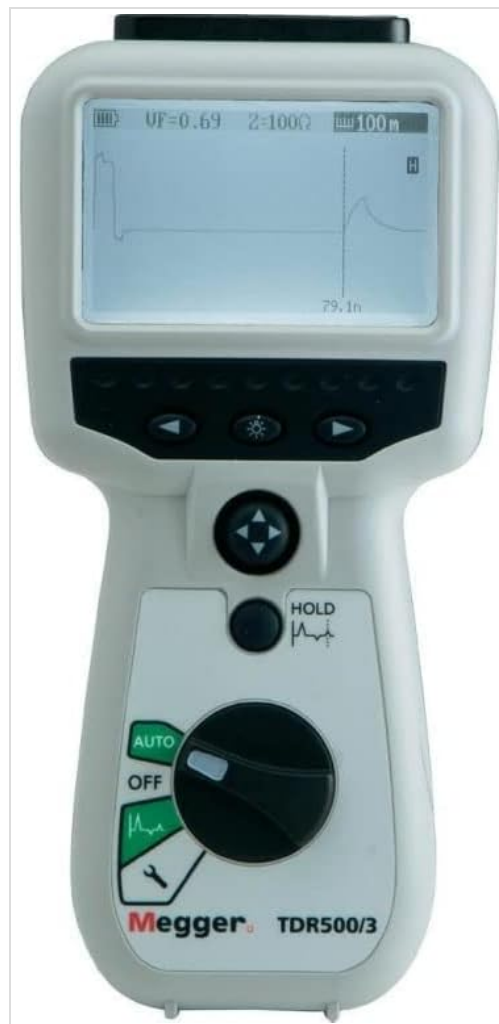
Figure 1: Front view of the Megger TDR500/3. The device features a monochrome LCD at the top, displaying trace data, velocity factor (VF), and impedance (Z). Below the screen are navigation buttons and a backlight control. A central four-way directional pad and a 'HOLD' button are located mid-body. The lower section includes a large rotary selector with 'AUTO', 'OFF', TDR waveform, and 'Setup' (wrench) positions, along with the Megger TDR500/3 branding.
