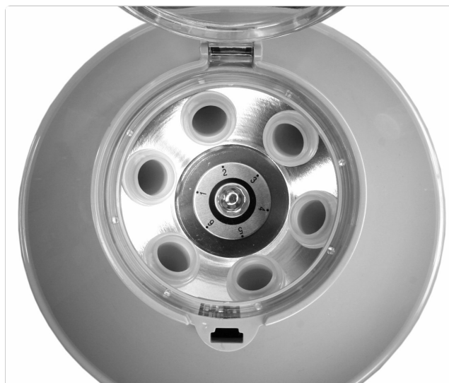
Figure 3: A close-up, top-down view of the fixed-angle rotor, showing the six numbered positions for sample tubes.
