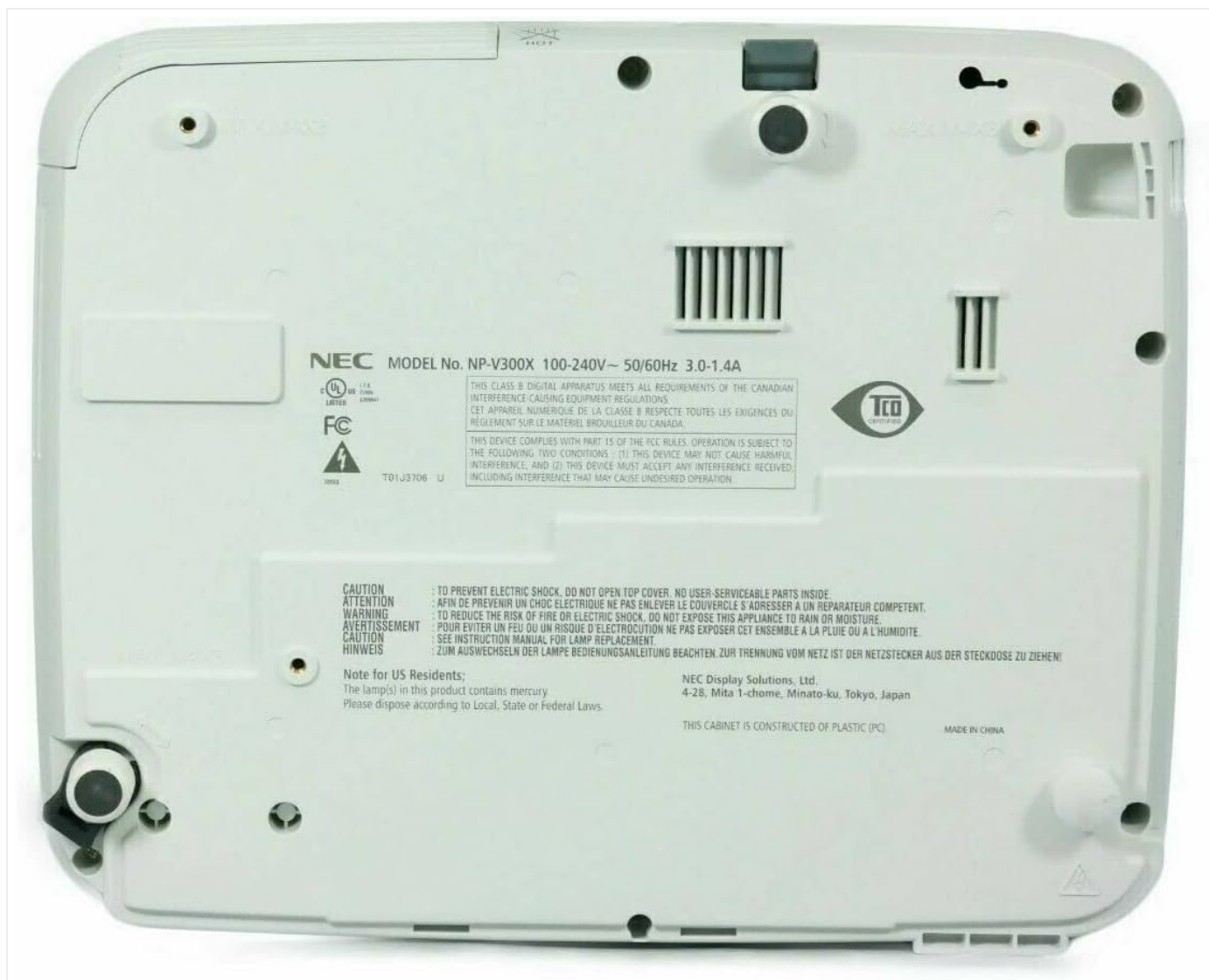
Figure 5: Bottom view of the NEC NP-V300X Data Projector, showing the model number (NP-V300X) and electrical ratings.
