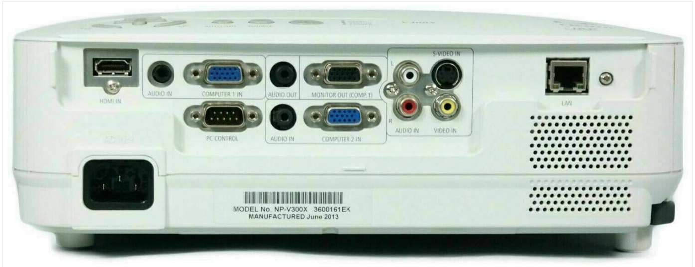
Figure 2: Rear panel of the NEC NP-V300X Data Projector, displaying various input and output ports including HDMI, VGA (COMPUTER 1 IN, COMPUTER 2 IN, MONITOR OUT), S-VIDEO IN, AUDIO IN/OUT, PC CONTROL, and LAN.
