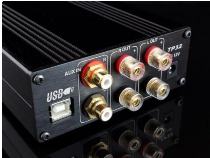
Image: Rear panel connections of the Topping TP-32EX. This view shows the USB B input, AUX IN (RCA), R OUT and L OUT speaker terminals, and the 12V DC power input.
