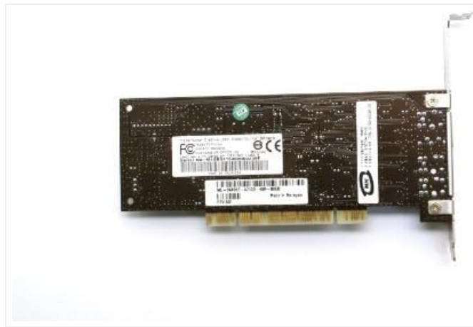
Figure 3: Underside view of the Creative Sound Blaster Live! SB0410, highlighting the PCI connector pins. This is the part that inserts into the motherboard's PCI slot.
