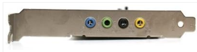
Figure 2: Rear panel view of the Creative Sound Blaster Live! SB0410, showing the various audio input and output ports. From left to right, these typically include line-out, line-in, microphone, and other surround sound outputs.
