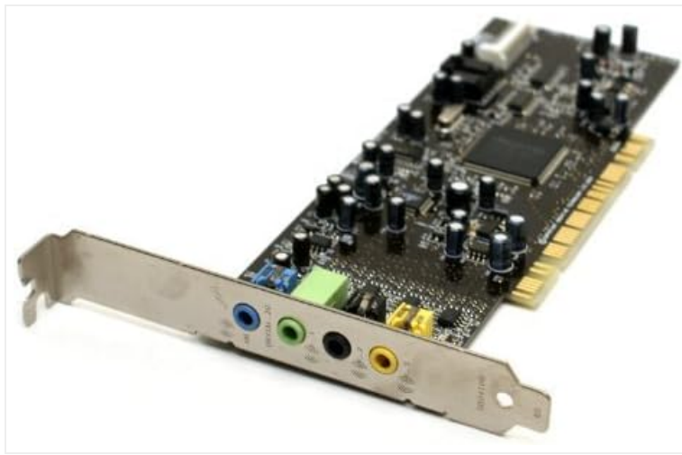
Figure 1: Top-down view of the Creative Sound Blaster Live! SB0410 PCI Sound Card. This image displays the overall layout of the circuit board, including various chips, capacitors, and the PCI connector at the bottom.
