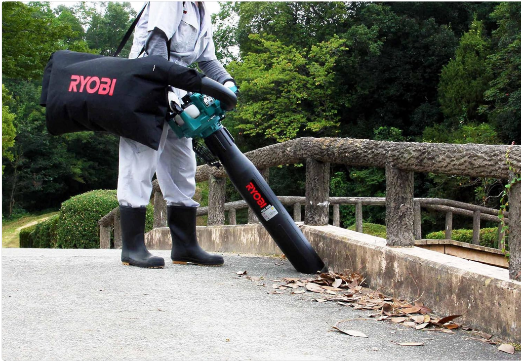
Image 5.3: A user operating the Kyocera EBVK-2650 in vacuum mode, actively collecting leaves from a paved area. The dust bag is visible, indicating collection.
