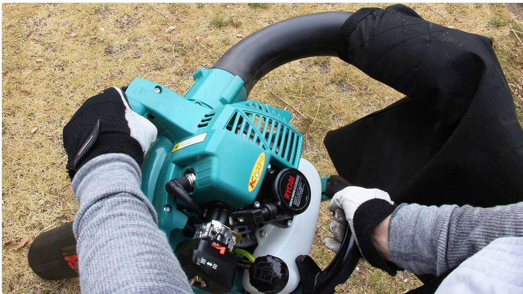
Image 4.2: The Kyocera EBVK-2650 being used in vacuum mode. The suction pipe is directed towards leaves, and the dust bag is visible, collecting the mulched debris.
