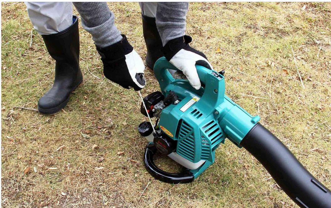
Image 5.1: A user demonstrating the engine starting procedure for the Kyocera EBVK-2650. The starter handle is being pulled to ignite the engine.
