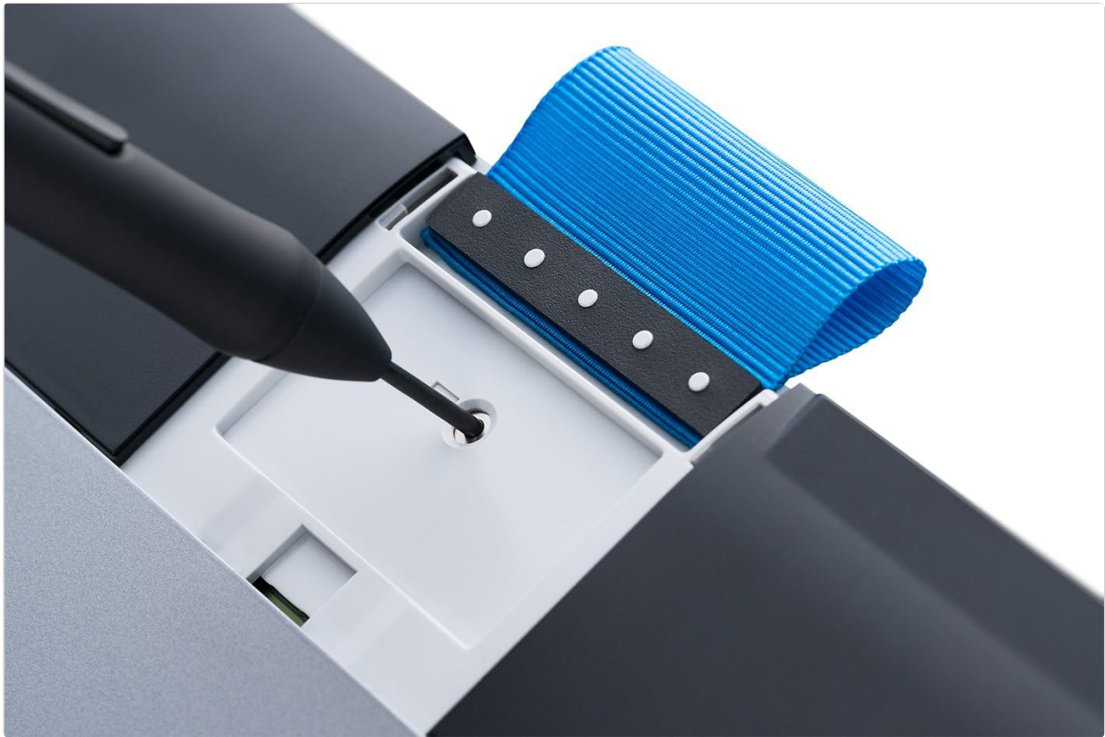
Image: A Wacom pen being used to remove a nib from the tablet, illustrating the nib replacement process.
