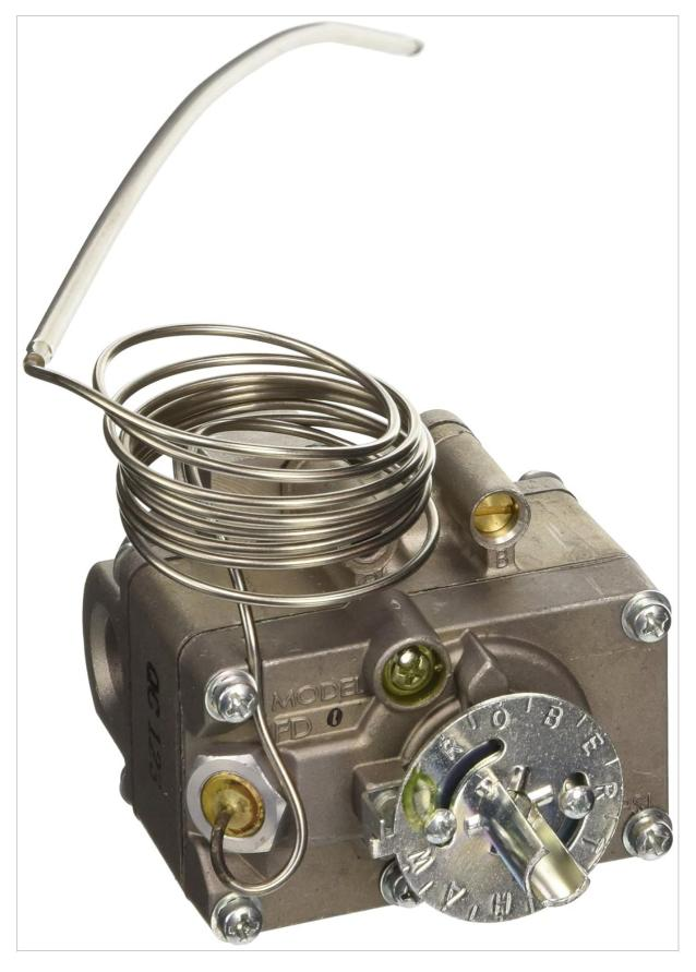
**Image Description:** A detailed view of the Garland G03145-048 Thermostat Control. The unit features a robust main control body, a coiled capillary tube, and a sensing bulb extending from the tube. The control dial, marked with various settings, is visible on the front face of the unit, secured by screws. The overall construction appears to be metal, indicating durability for commercial applications.
