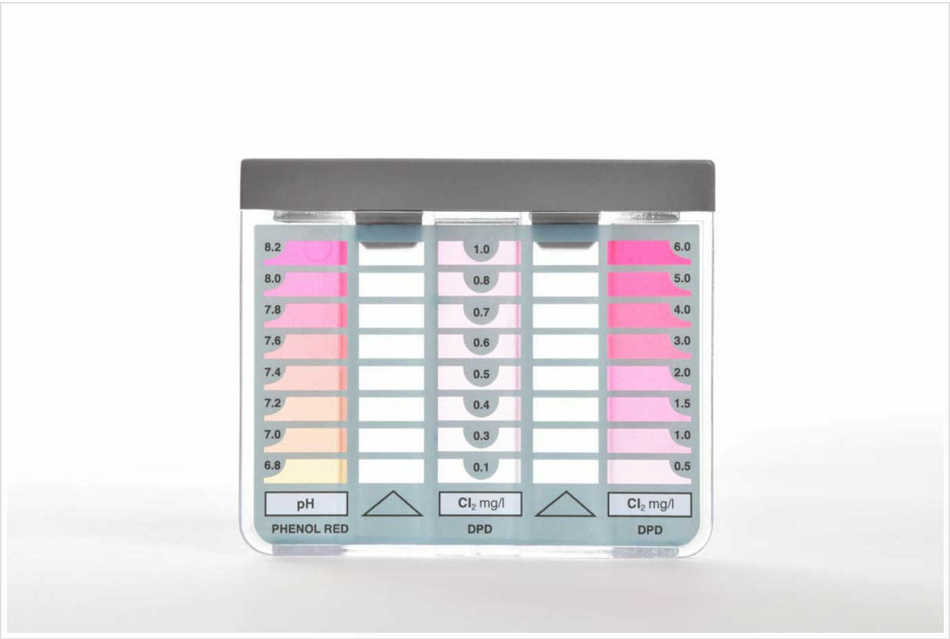
Figure 4: The transparent test block with distinct color scales for pH (left) and chlorine (right) measurements.
