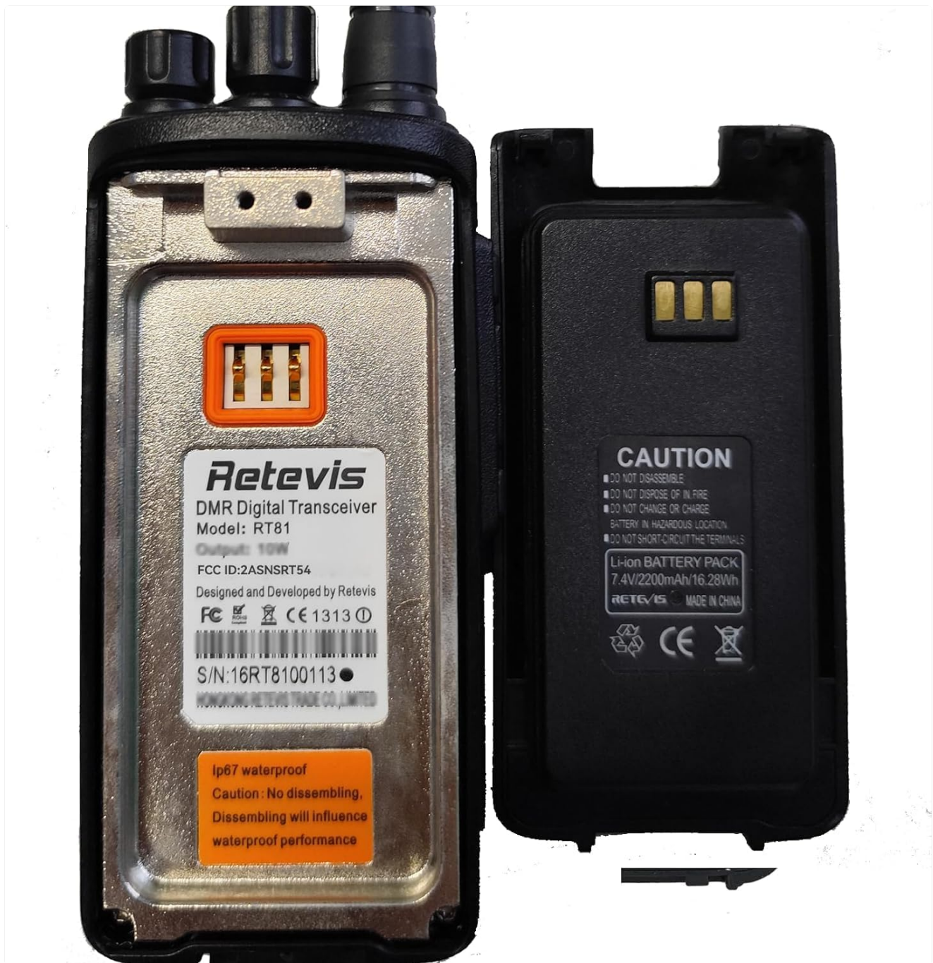
Figure 6: Battery Installation Area
