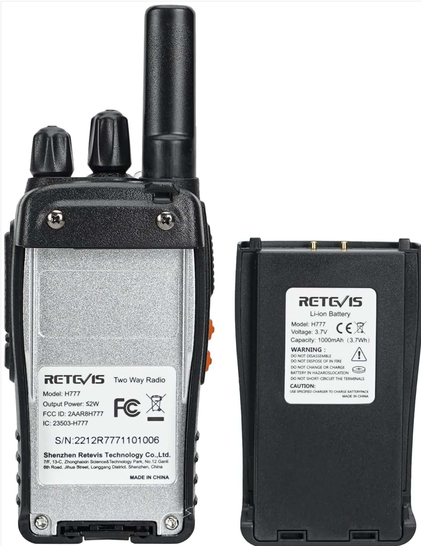
Image: The back of the Retevis H-777 radio and its removable Li-ion battery, showing how they connect.
