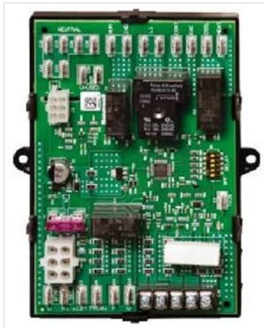
Figure 1: The Honeywell Furnace Control Circuit Board. This green circuit board features various electronic components, relays, and connection terminals, serving as the central control unit for furnace operations.
