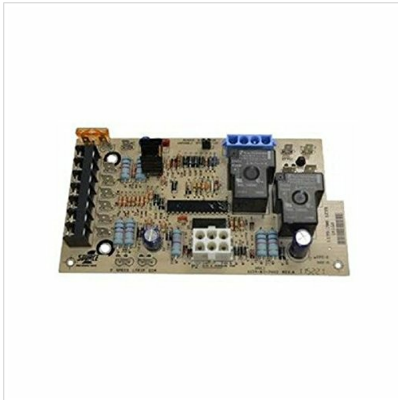
Figure 1: York Furnace Control Circuit Board S1-03101264002. This image displays the circuit board with various electronic components, connectors, and relays.
