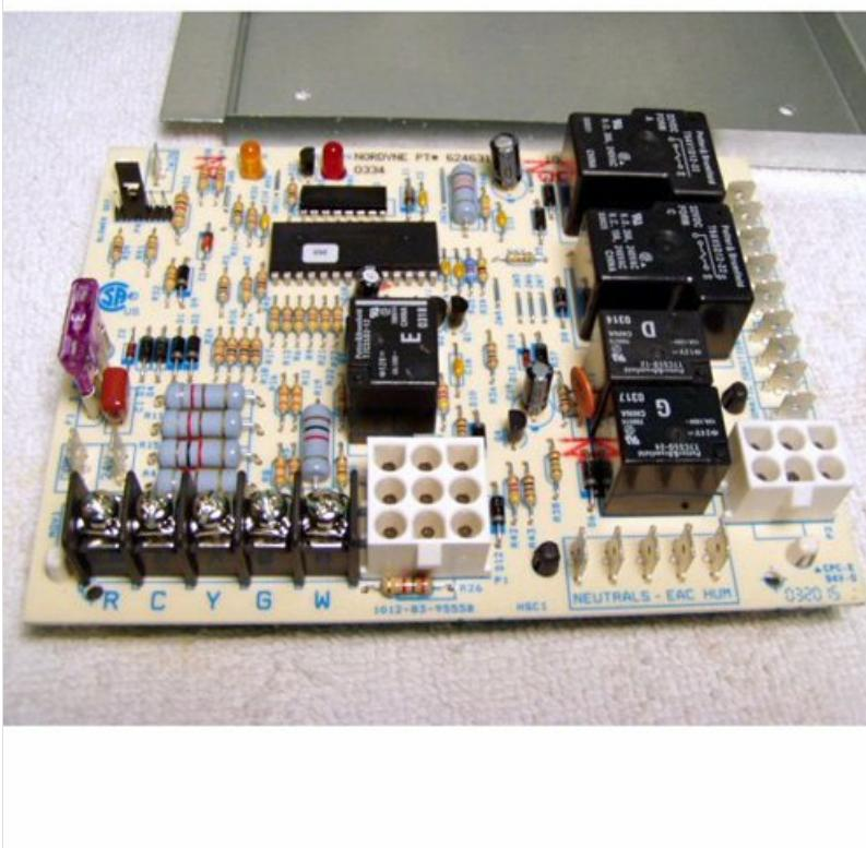
*Image showing the Nordyne OEM Upgraded Replacement Furnace Control Circuit Board, model 624591-0, with various connectors and components visible.*
