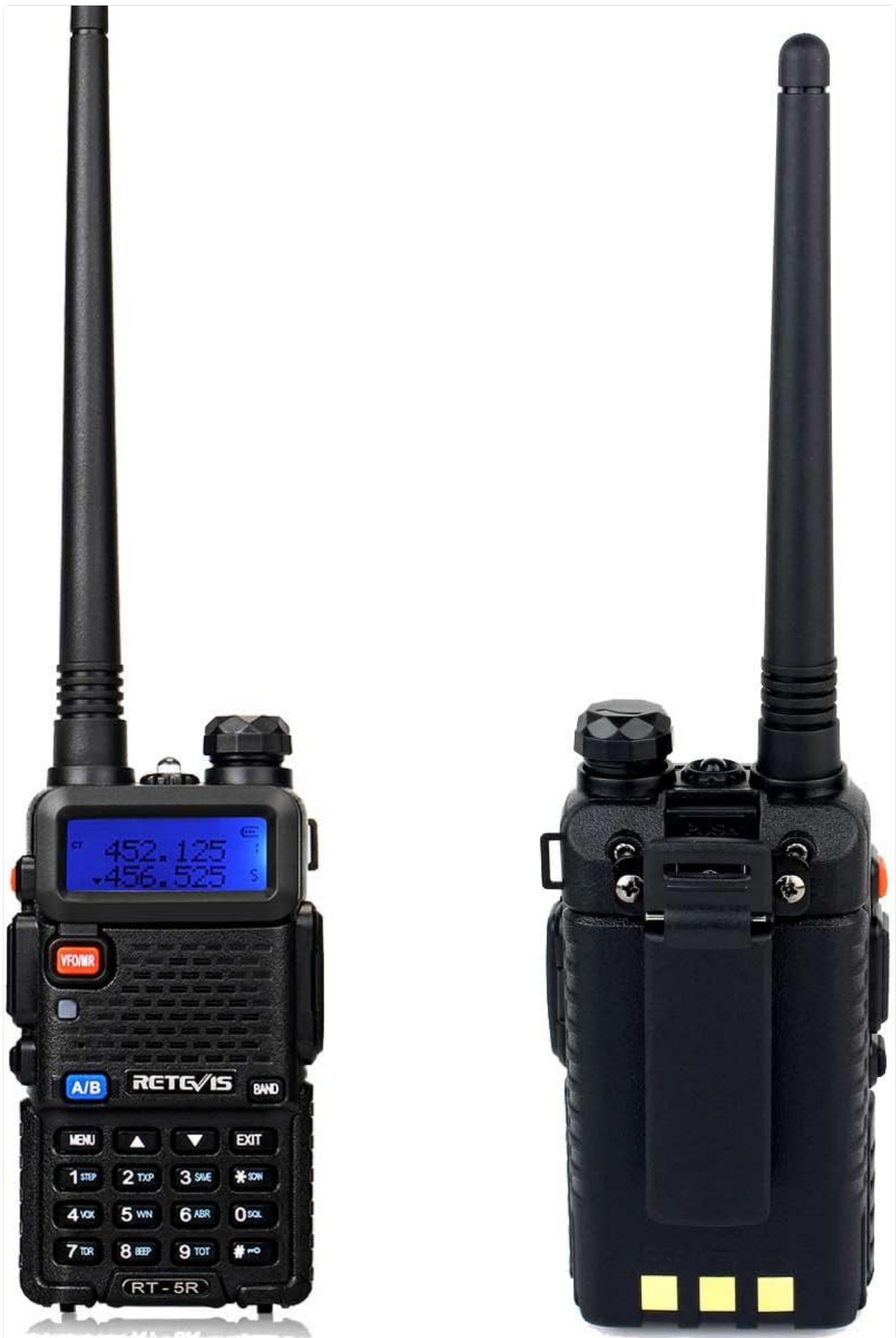
Image 3.1: Front and back view of the Retevis RT-5R radio, showing the display, keypad, PTT button, and belt clip attachment points.
