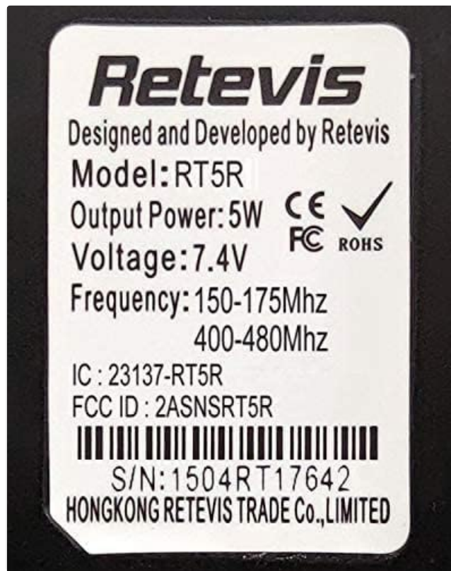
Image 8.1: Product label for the Retevis RT-5R, displaying model number, output power, voltage, frequency ranges, IC, and FCC ID.
