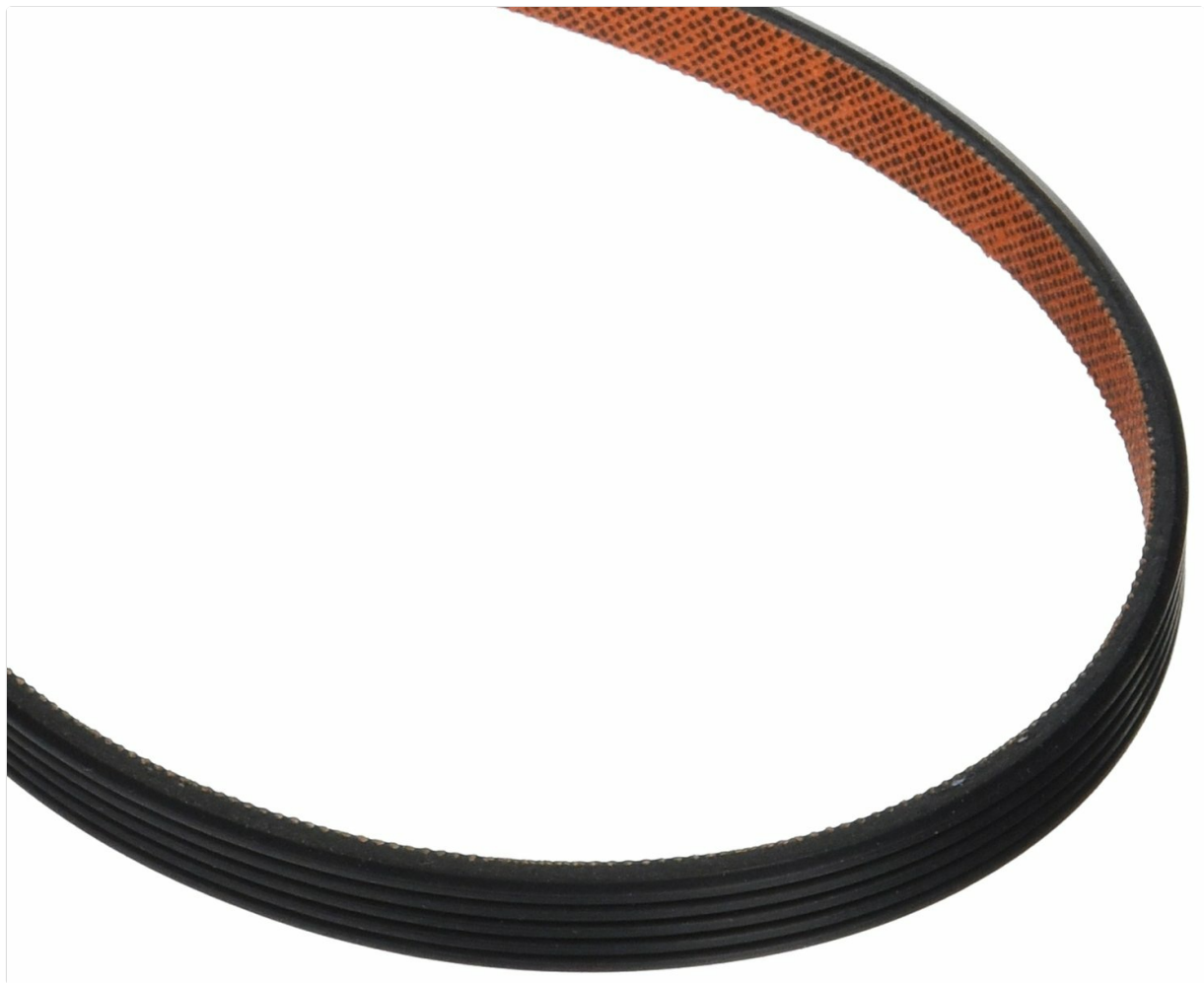
Image 1: The Whirlpool W10198086 Dryer Drum Belt. This image shows the ribbed side of the belt, which typically makes contact with the motor pulley and idler pulley, and the smooth side, which contacts the dryer drum.
