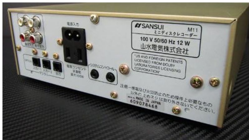
Image 2: Rear view of the SANSUI M11 Compact MD Recorder, showing the power input, RCA audio input/output, optical digital input/output, and system control ports.
