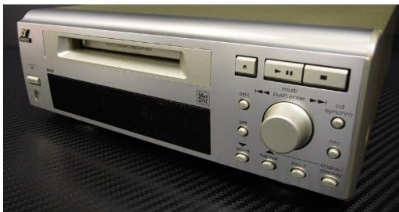
Image 1: Front view of the SANSUI M11 Compact MD Recorder, showing the MD slot, display, and control buttons such as Eject, Play/Pause, Stop, Multi-Push Enter knob, Record, Input, and Character/Display.
