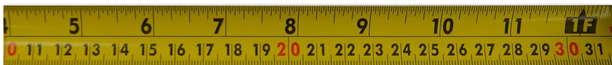
Image 3.2: A detailed view of the tape blade, showing both imperial (top row) and metric (bottom row) graduations for precise readings.
