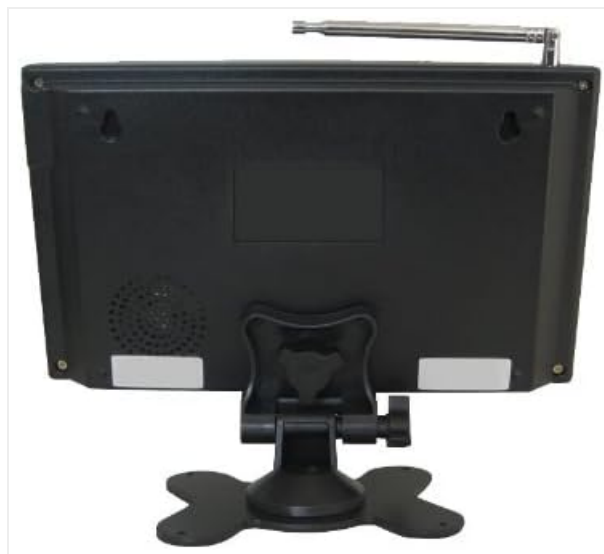
Figure 3.3: Rear view of the APE9500 receiver, showing the black casing, speaker grille, and mounting holes. A black adjustable stand is attached to the back, allowing for desktop placement or wall mounting.
