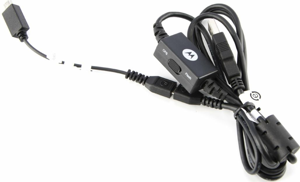
Image: The Motorola HKKN4027A programming cable features a switch to select between 'CPS' (Customer Programming Software) and 'Flash' modes. For general radio programming, ensure the switch is set to 'CPS'.
