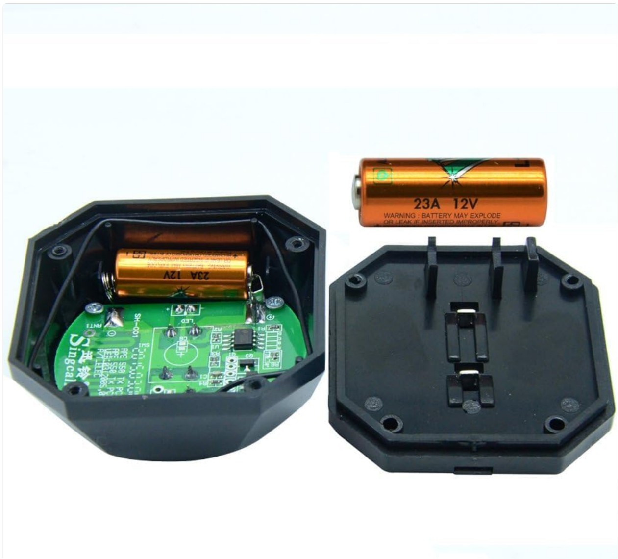
Image: The SINGCALL APE560 call button with its base removed, showing the battery compartment and a 23A 12V battery.
