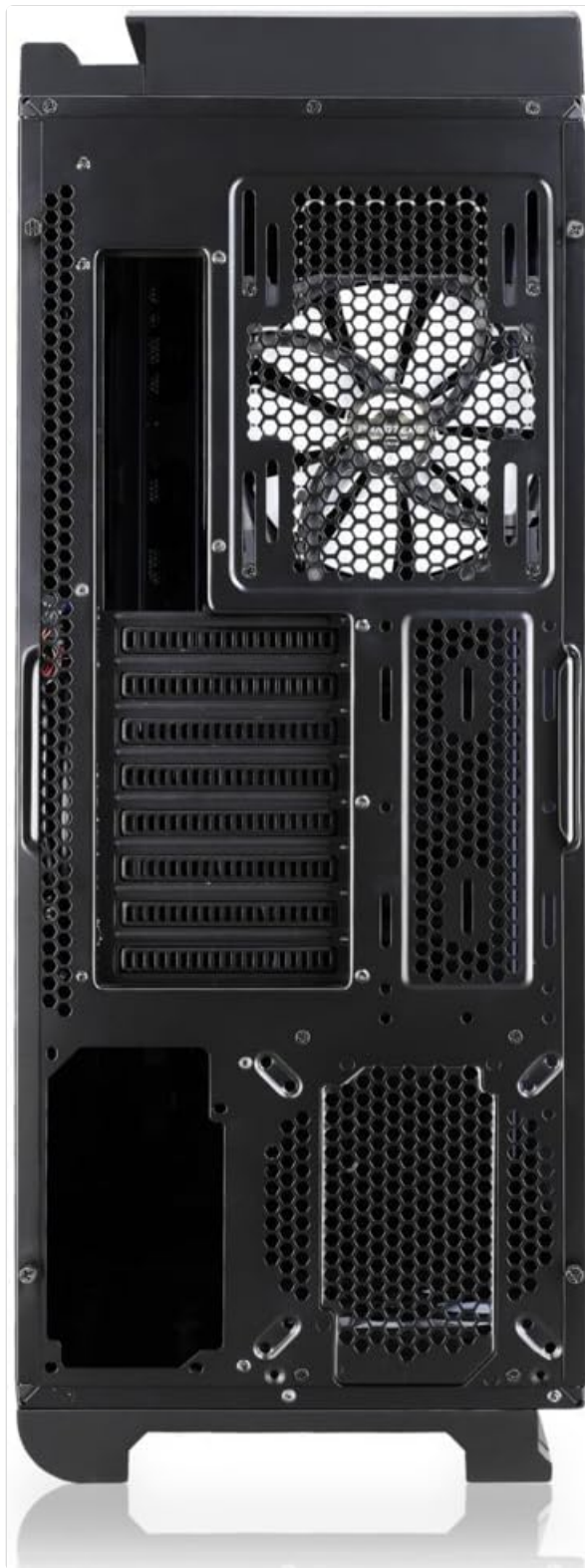
Figure 2: Rear view of the Enthoo Primo case, showing the PSU mounting area at the bottom.
