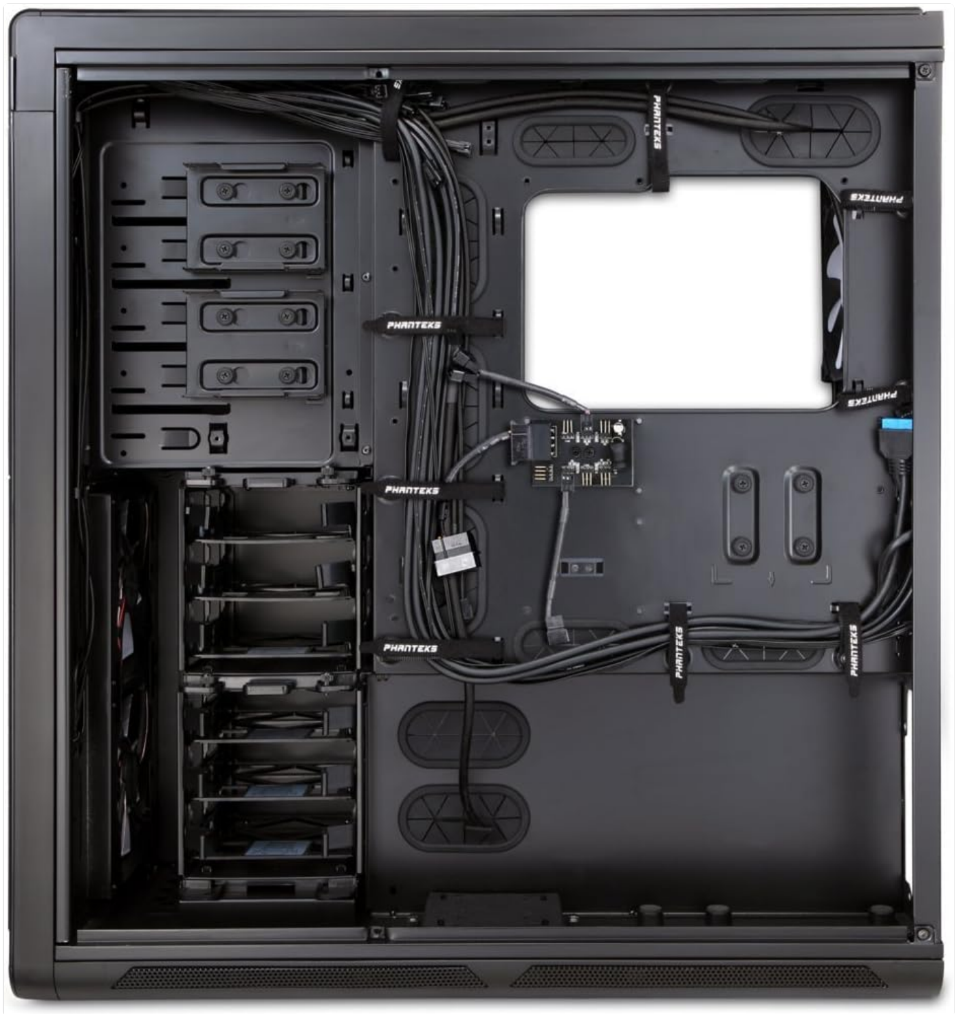
Figure 4: Interior view of the Enthoo Primo, showcasing the cable management features behind the motherboard tray.
