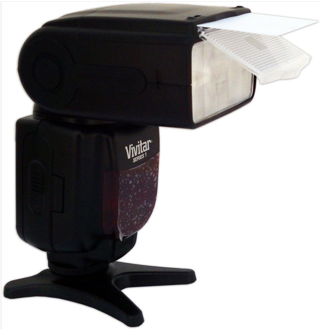
Image: Flash head with the bounce card extended, demonstrating its use for indirect lighting.
