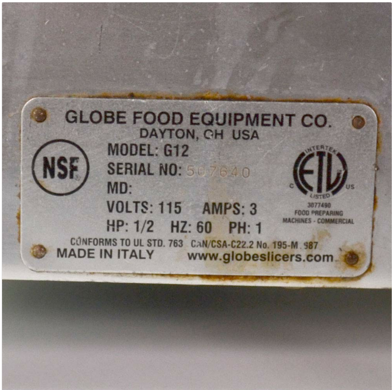
Figure 7.1: Close-up of the manufacturer's model plate, displaying key electrical and model specifications for the Globe G12 slicer.
