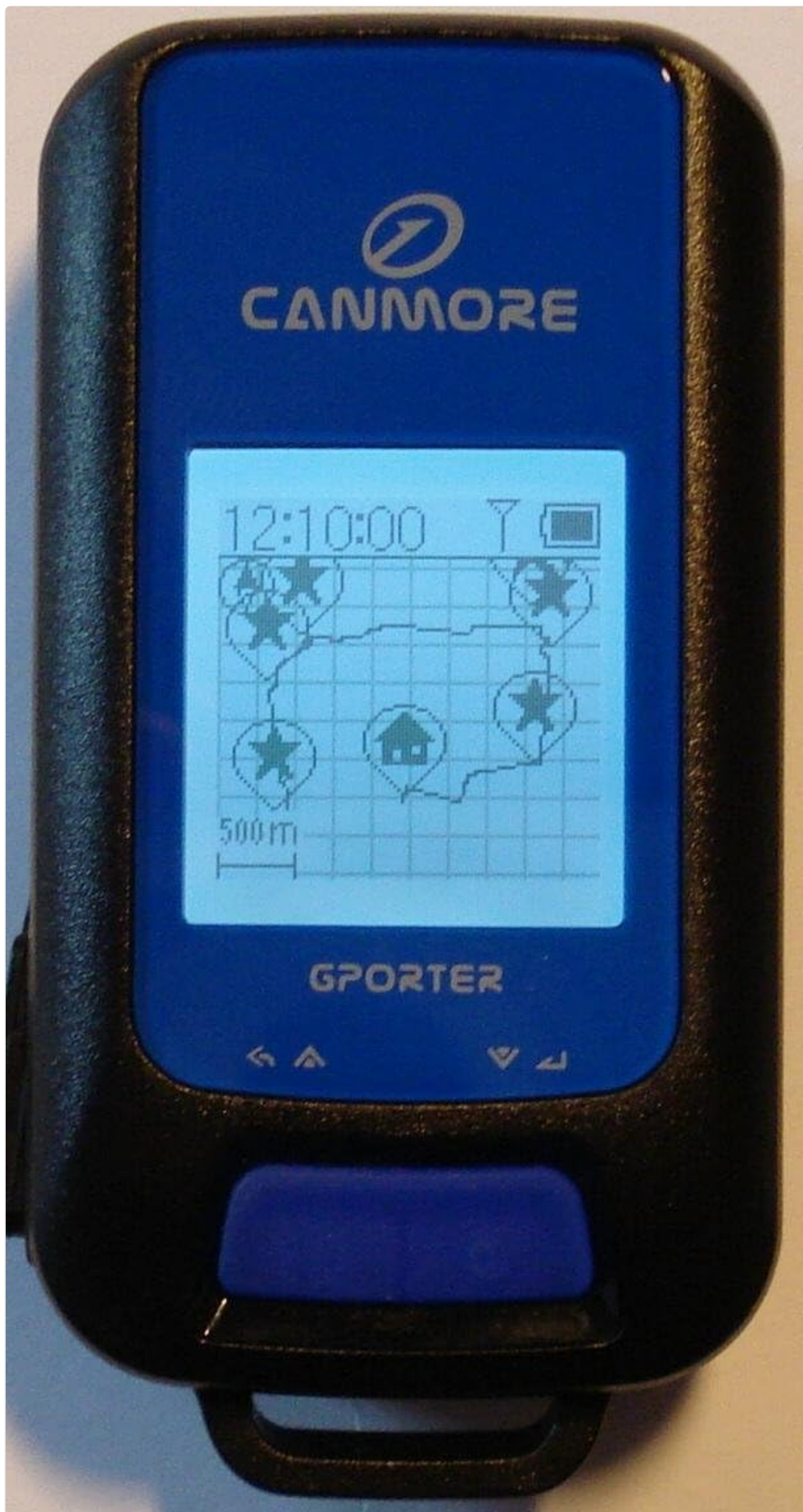
The device's screen is shown displaying a graphical representation of a recorded track or route. The display includes several waypoints marked with stars and a home icon, indicating navigation or tracking in progress.
