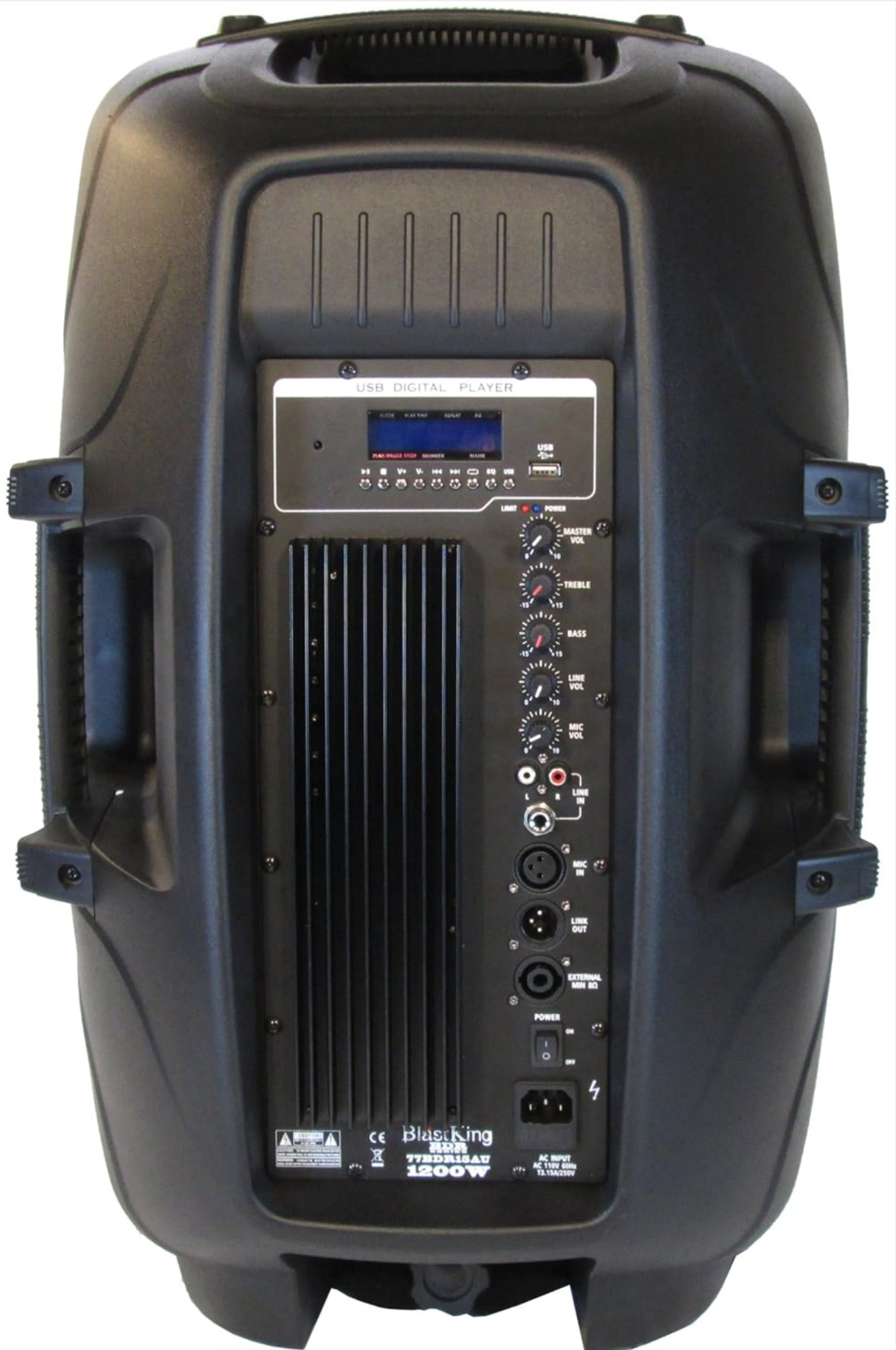
Image 3: Rear panel of the Blastking I77BDR15AU speaker. This view shows the comprehensive control interface, including the USB Digital Player, master volume, tone controls (treble, bass), microphone and line inputs, and power switch.
