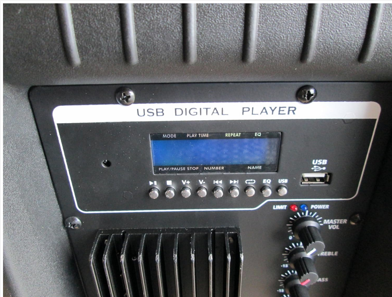
Image 4: Close-up of the USB Digital Player. This detailed view shows the LCD screen displaying mode, play time, repeat status, and EQ settings. Below the screen are control buttons for play/pause, volume/track skip, mode, repeat, and EQ, along with a USB port.
