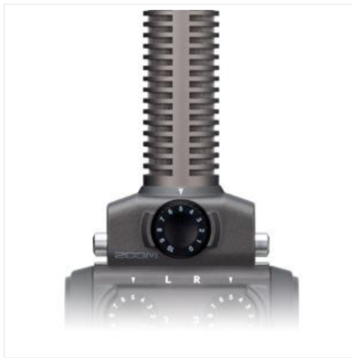
Figure 2: EXH-6 capsule securely attached to a Zoom H6 Handy Recorder.
