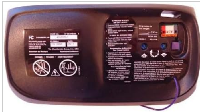
Image: Back of the LiftMaster 41AS050-1 Receiver Logic Board. This view displays the part number (41AS050-1), FCC compliance information, and detailed instructions for programming new remote controls and erasing all existing remote codes. Key elements include wire terminals for connection and a "SMART" button for programming.
