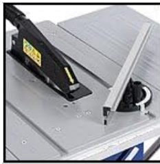
Image 3.2: Detail of the blade guard and rip fence. This view shows the transparent blade guard covering the saw blade, the splitter behind the blade, and the adjustable rip fence positioned on the table surface.
