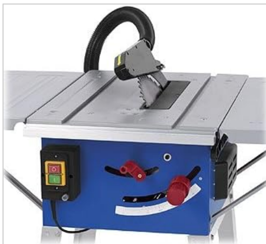
Image 3.1: Close-up of the control panel and blade adjustment mechanisms. This image highlights the power switch (green for ON, red for OFF), the red knob for blade height adjustment, and the red lever for blade bevel angle adjustment, along with the angle scale.
