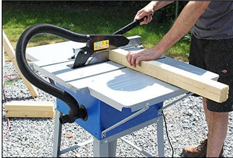
Image 5.1: Table saw in use, demonstrating a cutting operation. This image shows a user guiding a wooden workpiece through the saw blade, with the dust extraction hose visible and sawdust being produced.
