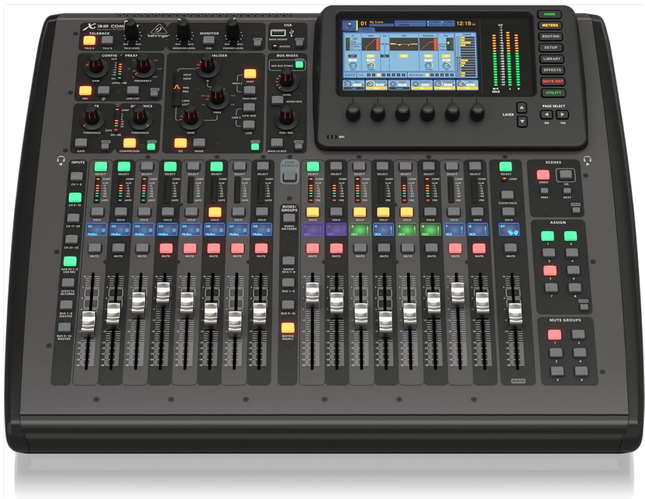
Figure 3: Angled front view of the Behringer X32 Compact, highlighting the motorized faders and LCD scribble strips.
