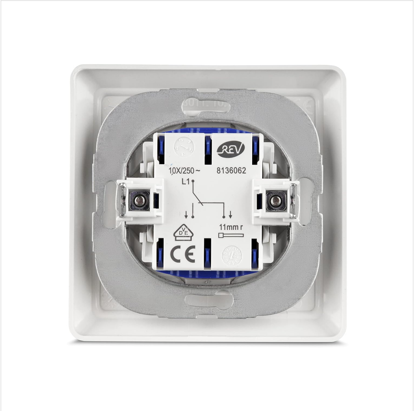
Image 5.1: Rear view of the switch mechanism with wiring terminals. L1 indicates the live input, and the arrows indicate output terminals for two-way switching.
