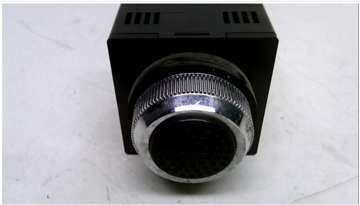
Figure 2: Close-up of Speaker Grille. A detailed view of the signal phone's speaker grille, showing its textured surface and the metallic, finely ribbed bezel that secures it to the device housing.
