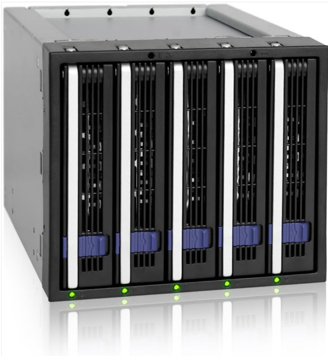
Figure 4.1: Front view of the MB155SP-B unit, showing its five drive bays.
