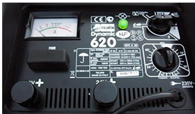
Figure 2: Close-up of the control panel, detailing the ammeter, voltage and charge mode selectors, and the timer function.
