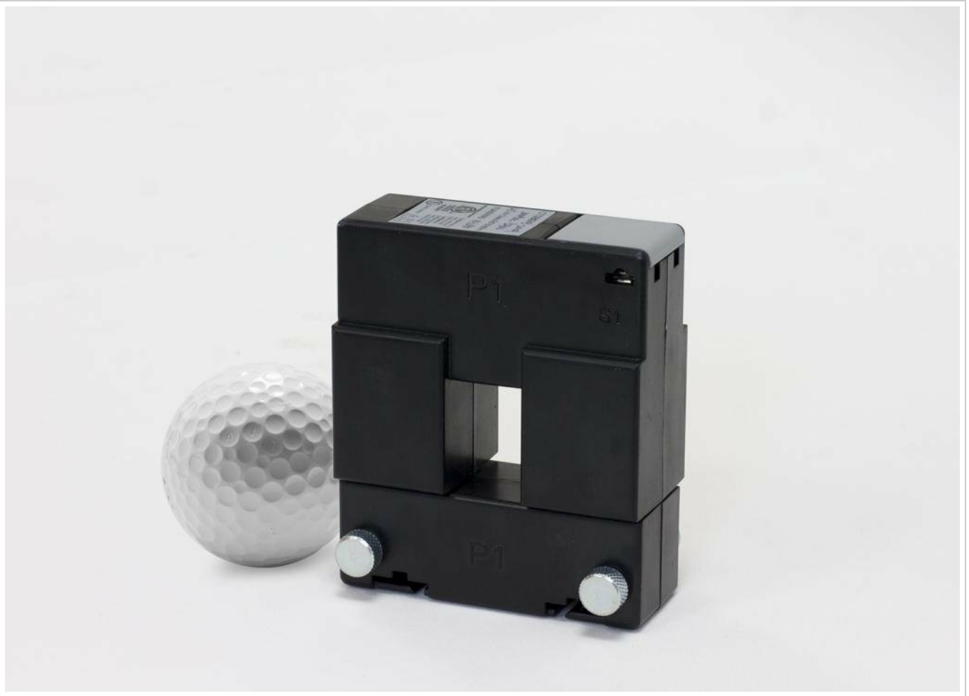
Figure 3.1: Accuenergy AcuCT-0812-200:5 Split-Core Current Transformer. The image shows the black, rectangular split-core current transformer with its two halves joined, next to a white golf ball for size comparison. The transformer has visible markings "P1" and "S1" on its casing.
