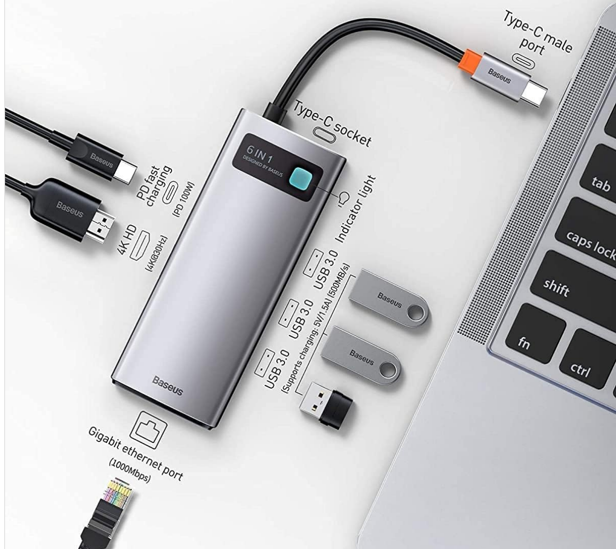
Image: The Baseus Metal Gleam USB-C Hub showcasing its various ports including USB-C, HDMI, USB 3.0, and Ethernet.
