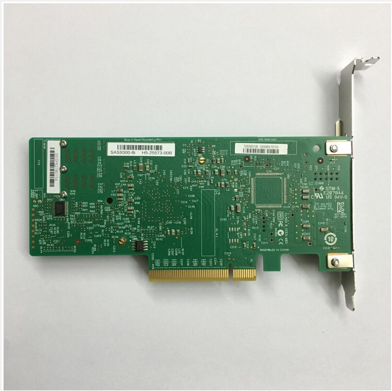
This image displays the LSI Broadcom SAS 9300-8i Host Bus Adapter, highlighting its circuit board components, SAS9300-8i model designation, and H5-25573-00 part number. Key features visible include the SFF-8643 mini-SAS HD internal connectors and the PCIe Express interface.
