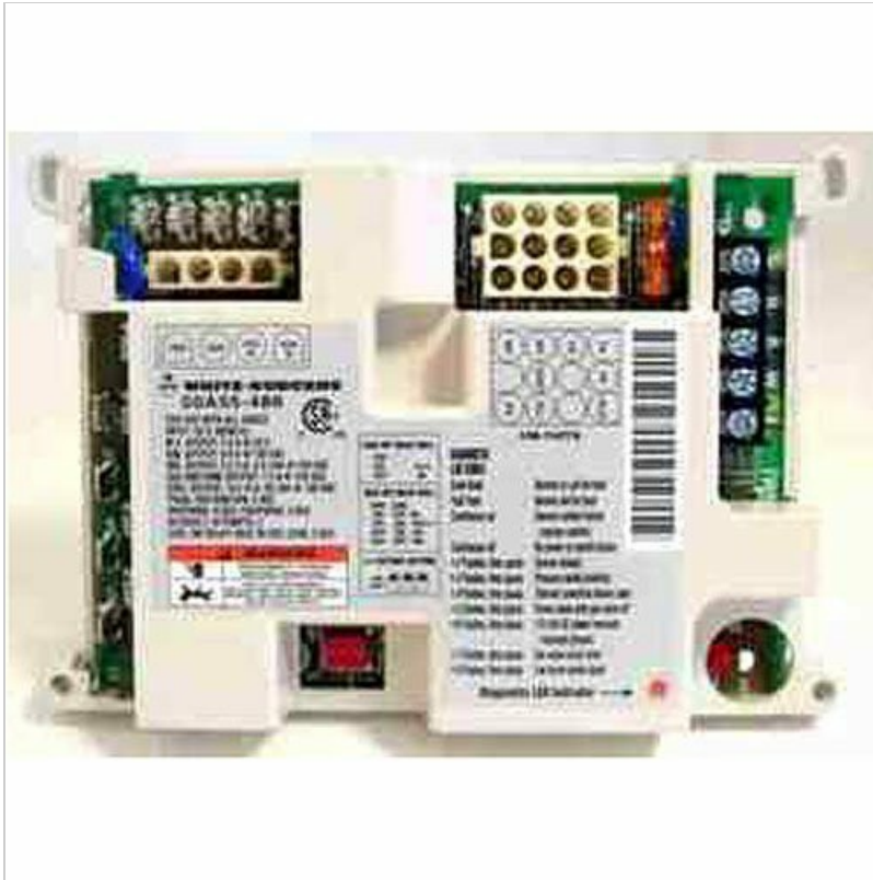
Image: The Trane White Rodgers Upgraded Furnace Control Circuit Board, model D341122P01, showing various terminals and components. This image provides a visual reference for the board's layout during installation.
