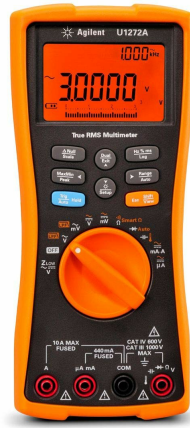
Figure 3.1: Front view of the U1272A multimeter, showing the OLED display, function dial, and input terminals.
