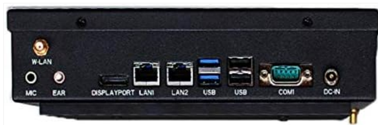
Image 2: Rear view of the Touch-PC, highlighting the various input/output ports. From left to right: W-LAN antenna connector, Microphone input, Earphone output, DisplayPort, LAN1, LAN2, USB 3.0 ports (blue), USB 2.0 ports, COM port (DB9), and DC-IN power input.
