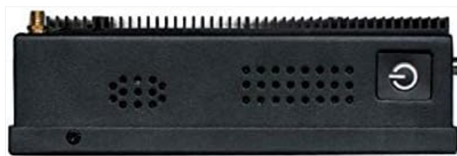
Image 3: Side view of the Touch-PC, showing the power button and additional ventilation grilles.
