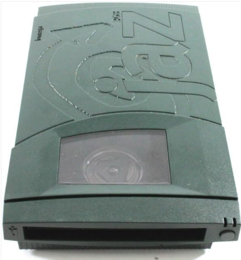
Image: Front view of the Iomega Jaz V2000S drive, showing the disk insertion slot and eject button.
