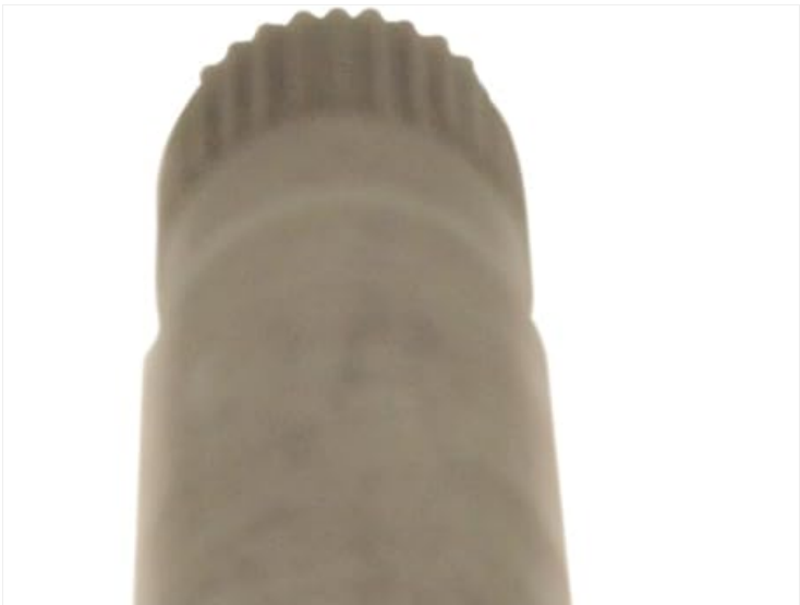
Figure 1: Side view of the Spicer 45531 Front Axle Shaft, showing its cylindrical shape and splined ends for connection to the differential and wheel hub.
