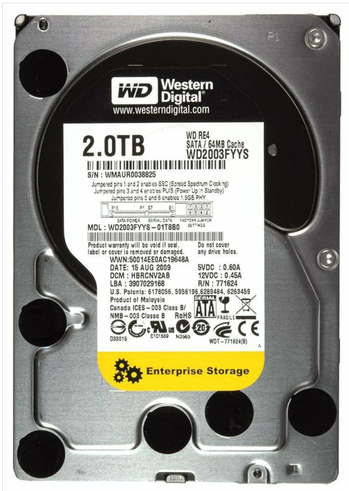
Figure 1: Western Digital WD2003FYYS 2TB Internal Hard Drive. This image displays the typical appearance of the hard drive, featuring a rectangular metal enclosure with a circuit board on the underside and standard SATA data and power connectors at one end.
